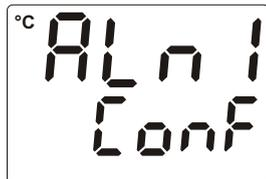
6 - If user does not do anything for 120 seconds while device is on technician menus, device turns to operation screen.
